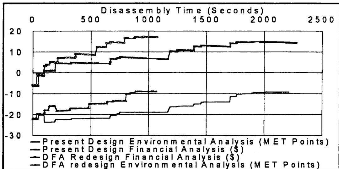
Figure 4 Disassembly analyses of an automatic washing machine
