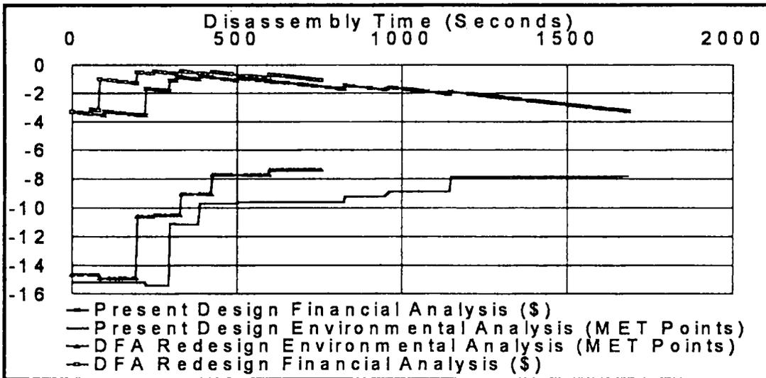
Figure 6 Disassembly analyses of a color TV set
