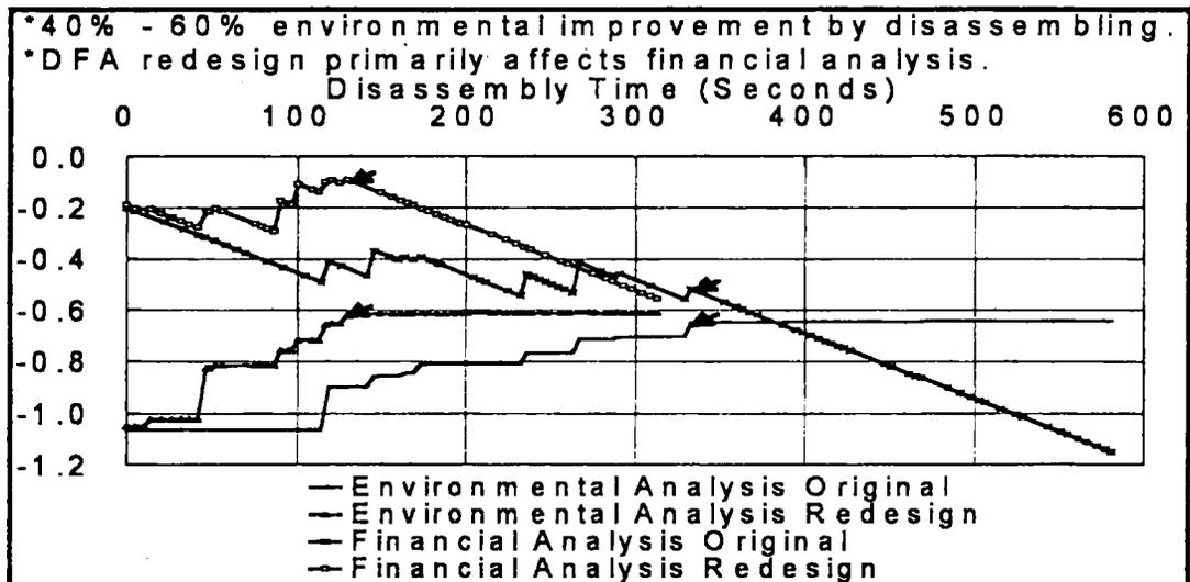
Figure 3 Disassembly analyses of original and redesigned coffee maker
