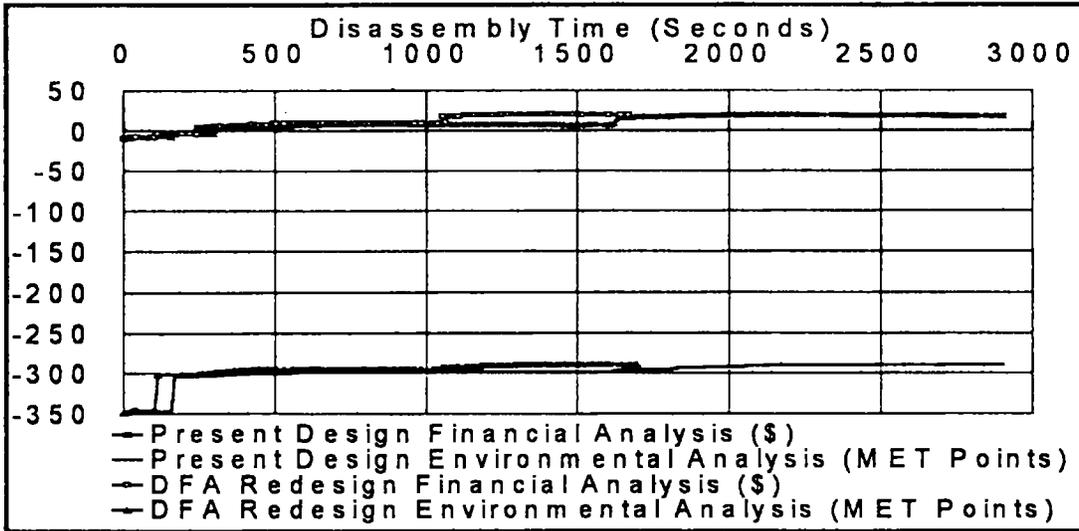
Figure 5 Disassembly analyses of a refrigerator
