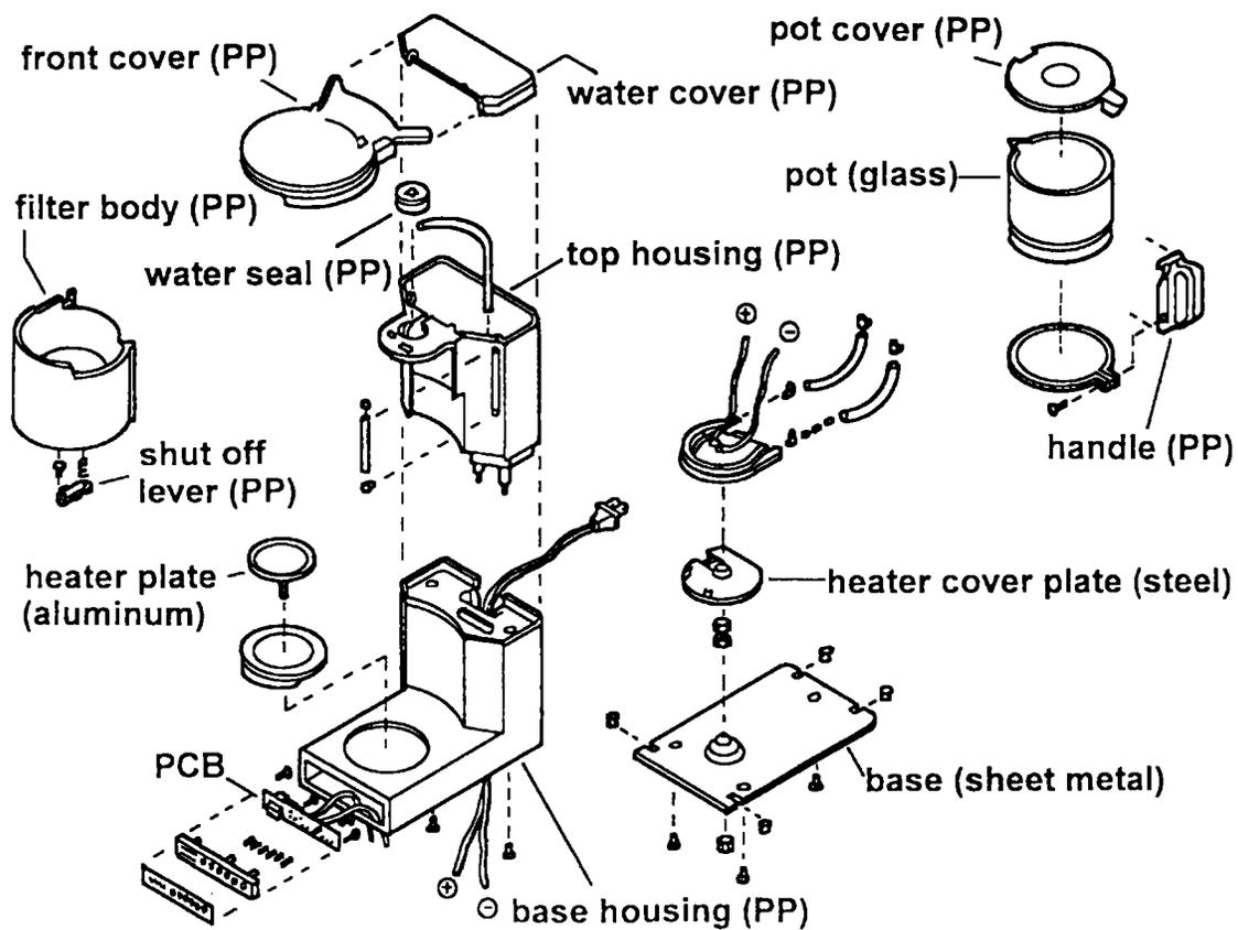
Figure 1 Exploded view of coffee maker
