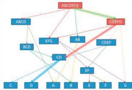
Fig 4: AND/OR disassembly representation. Red assembly represents OR node with dual AND output
