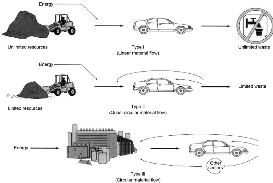
Fig. 5. Vehicle recycling models [47].
