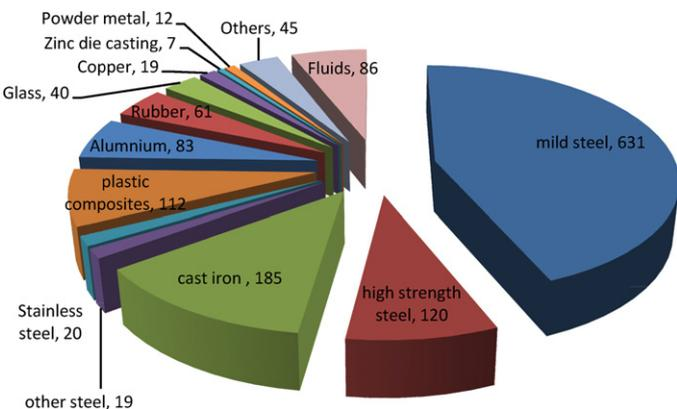
Fig. 9. Material distribution of total vehicle curb weight in kg [50].
