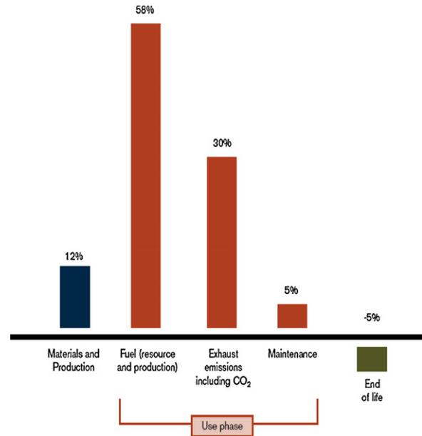
Fig. 14. Distribution of the environmental impact from a Volvo FH truck in long-haul operation [74].
