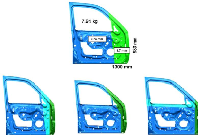
Fig. 6. Tailor welded blank applied for door inner [50].
