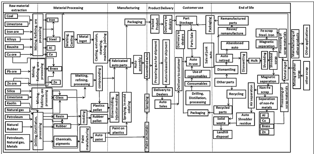
Fig. 3. Detailed LCA for materials used, manufacturing processes and end-of-life scenarios [50].
