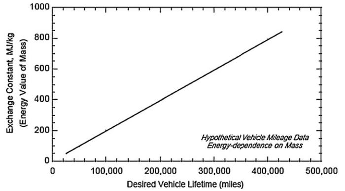
Fig. 11. Approximated relationship between vehicle mass and lifetime energy consumption, computed as a function of vehicle lifetime in miles [83].
