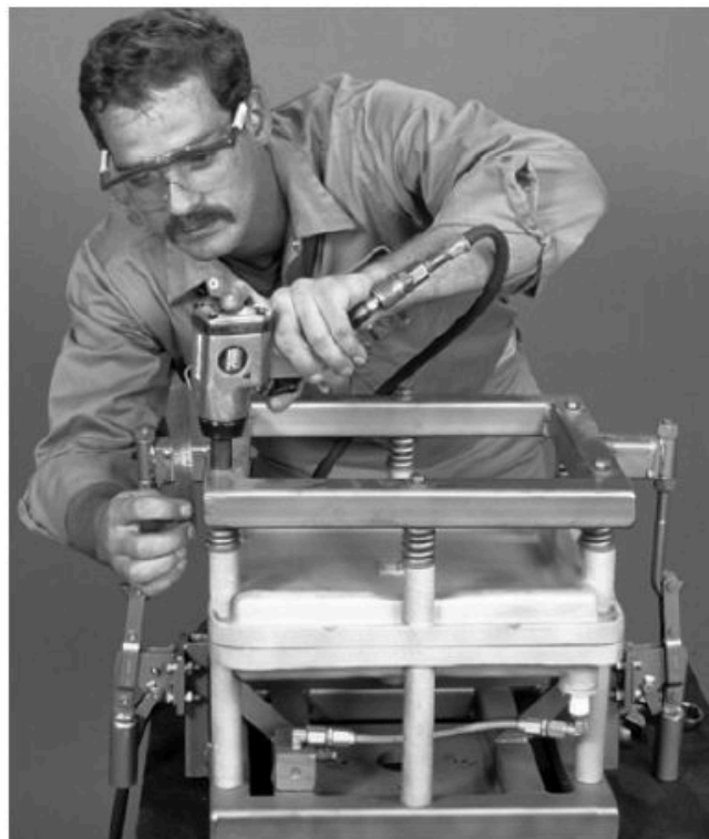
FIGURE 6.14 Fitting and adjustment of a frame for spring tension on a cast aluminium mold. (Courtesy of Wheeler Boyce, Inc.)
