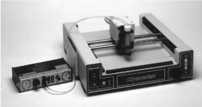
FIGURE 9.10 EFD dispenser and Asymtek benchtop system. (Courtesy of Asymtek.)
