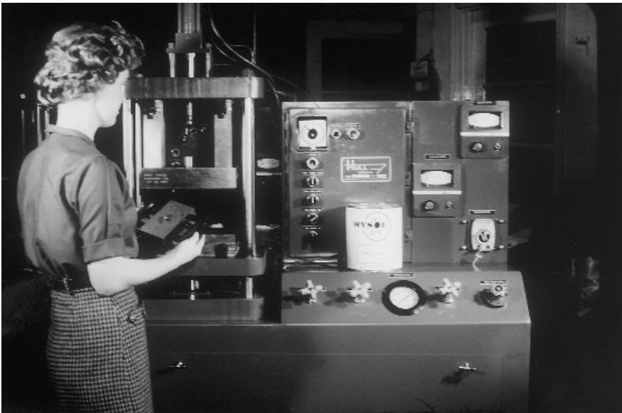
FIGURE 7.12 Transfer press for laboratory development and modest production. Note the hand mold for inexpensive pilot production of small parts.
