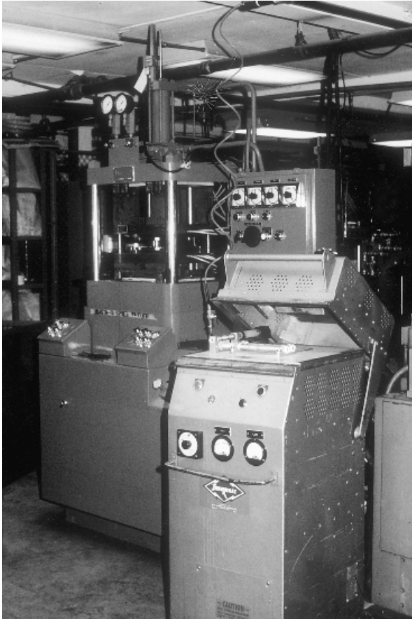
FIGURE 7.5 A high-frequency preheater, positioned next to the press, enables faster cures for both transfer and compression molding.
