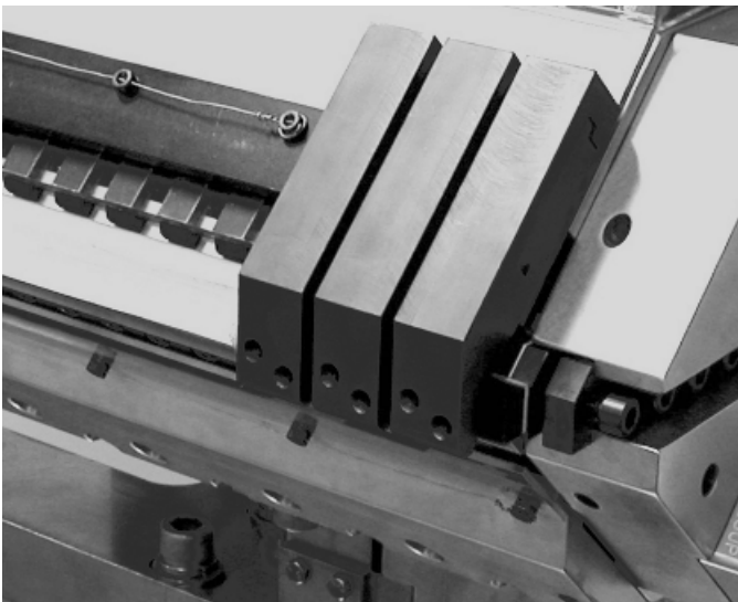
FIGURE 3.19 Fixed-side exterior deckle assembly. (Courtesy of EDI, Chippewa Falls, WI.)
