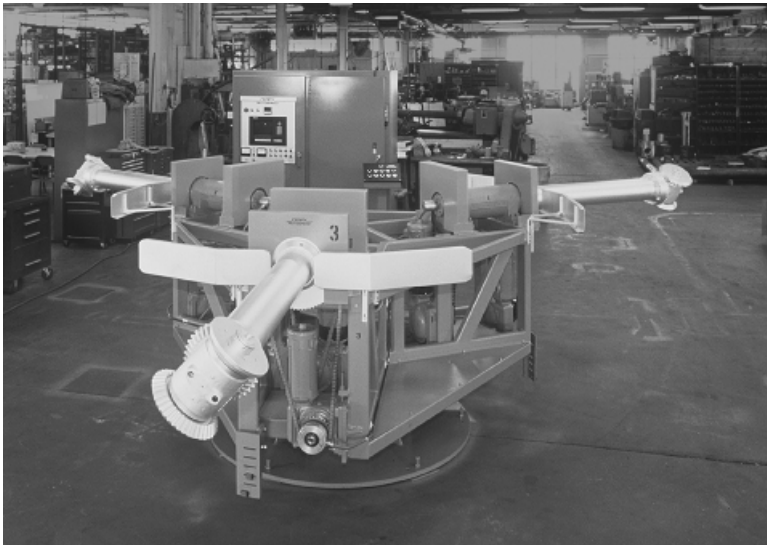
FIGURE 6.26 Center assembly for a three-arm turret machine. (Courtesy of Ferry Industries, Inc.)
