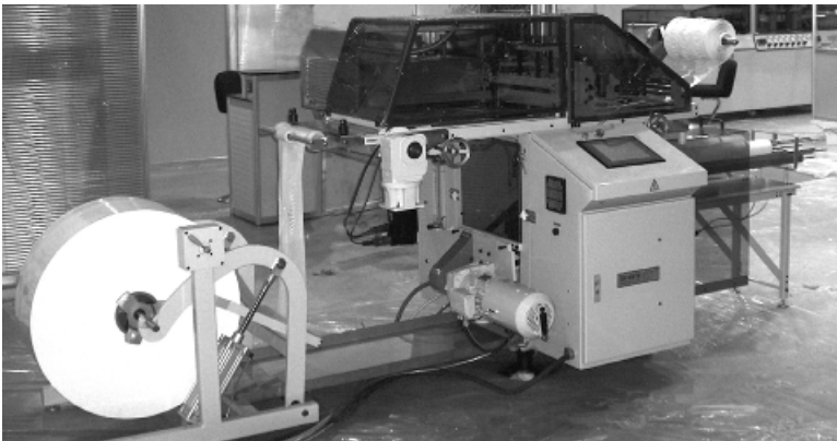
FIGURE 3.64 Roll-fed thermoformer. (Courtesy of G. N. Plastics Company Limited, Chester, Nova Scotia, Canada.)
