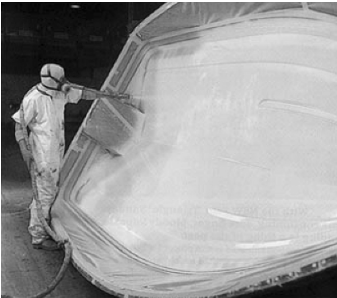
FIGURE 8.9 Spray-up technique. (Courtesy of Owens Corning. Used with permission.)
