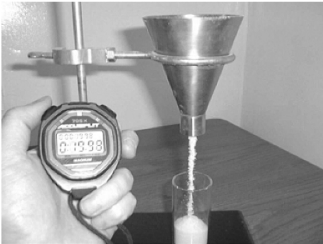
FIGURE 6.11 Free-flowing powder during a flow rate test.
