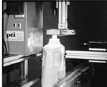
FIGURE 5.63 (a) Camera-based vision inspection system for plastic containers; (b) scanning bottle labels for unacceptable skew; (c) scanning bottlenecks for defects related to thread profile, neck slant, flash, and neck diameter, and height. [(a) Courtesy of Cognacs Corp., Natick, MA; (b) and (c) courtesy of Packaging Technologies and Inspection, Tuckahoe, NY.]
