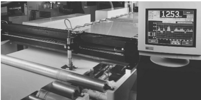
FIGURE 3.45 Gamma backscatter in scanning operation. (Courtesy of NDC, Irwindale, CA.)
