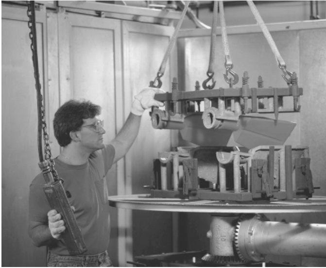
FIGURE 6.21 Servicing (demolding) station at ground level. (Courtesy of Ferry Industries, Inc.)
