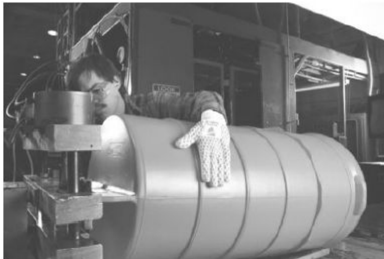
FIGURE 5.58 Finishing an extrusion blow-molded traffic safety barrel. (Courtesy of Crocker Ltd., Three Rivers, MI.)
