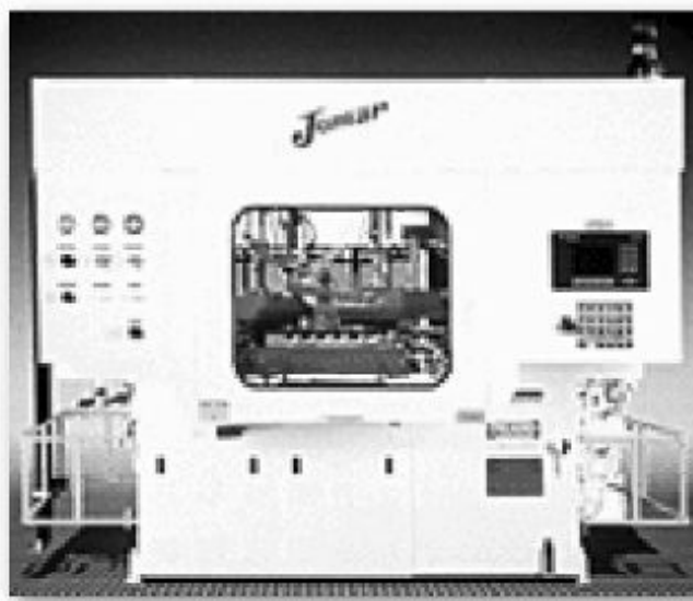
FIGURE 5.17 Injection blow molding machine. (Courtesy of Jomar Corporation.)
