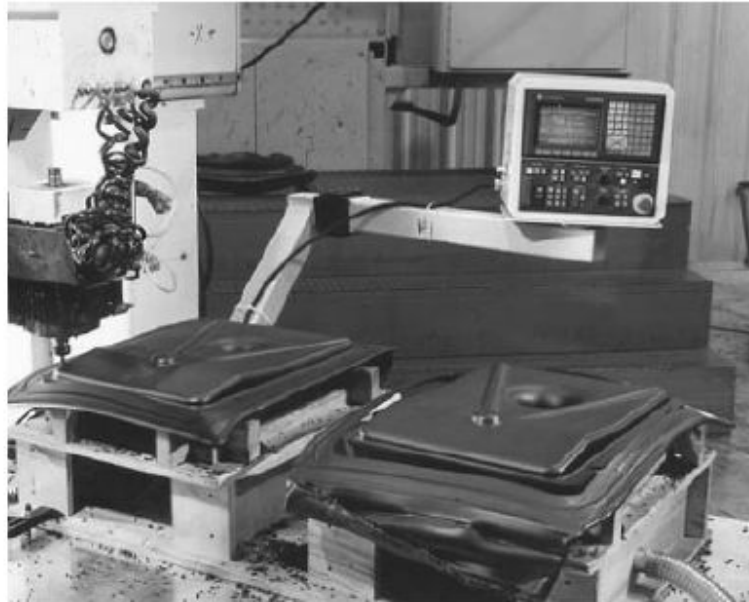
FIGURE 5.61 Using a CNC router to trim blow-molded panels automatically. (Courtesy of Agri-Industrial Plastics, Fairfield, IA.)
