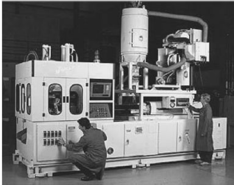
FIGURE 5.22 Injection stretch blow molding machine manufactured by Jomar Corporation, Pleasantville, NJ.
