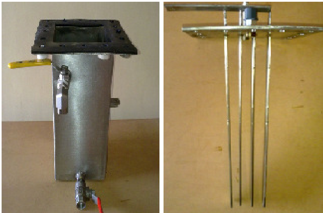
Figure 2. Arrangements of electrodes in second design of electrolyser.
