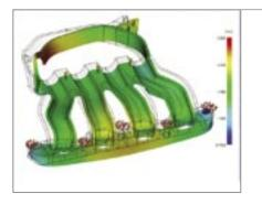
**MPI/Stress** predicts the post-molding performance of plastic parts when subject to various forms of external loading. The analysis considers the effects of plastic flow during injection molding and the resultant mechanical properties on the component's structural integrity.
