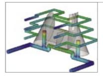
**MPI/Cool** provides tools for modeling mold cooling circuits, inserts, and bases around a part and analyzing the efficiency of the mold's cooling system. MPI/Cool simulations allow users to optimize mold and cooling circuit design to achieve uniform part cooling, minimize cycle times, eliminate part warpage due to cooling factors, and decrease overall manufacturing costs.
