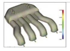
**MPI/Fiber** helps predict the fiber orientation due to flow in fiberfilled plastics and the resultant mechanical strength of the plastic/fiber composite. It is important to understand and control the orientation of fibers within fiber-filled plastics to reduce shrinkage variations across the molded part to minimize or eliminate part warpage.
