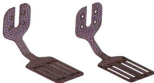
CAD geometry meshed with solid elements
