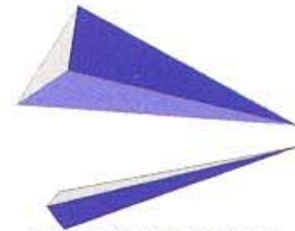
Excessively distorted elements
